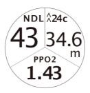
Under water mode Exceed PPO2 settings Shows PPO2 and flashing.
