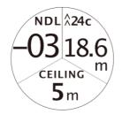
Under water mode Exceed NDL Shows Ceiling Depth When reach the ceiling shows the stop time by counting down
